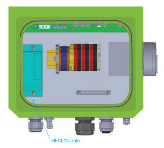
Figure 29: Internal View of Cell\_GFCI
