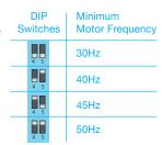
• NOTE: The Cell 3500's default minimum Hz setting is 30Hz.
