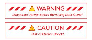
Before performing any service or maintenance inside the controller or when connecting or disconnecting any wires, **DISCONNECT the power** and **WAIT 90 seconds** to allow the capacitor bank inside the controller to discharge to a level below 50V.
